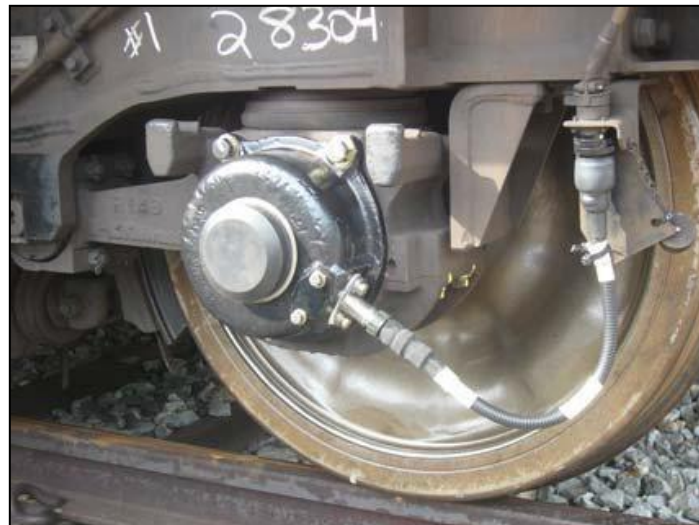
Figure 22: Tachometer Installed to Train Wheel (Sin, 2013a)
