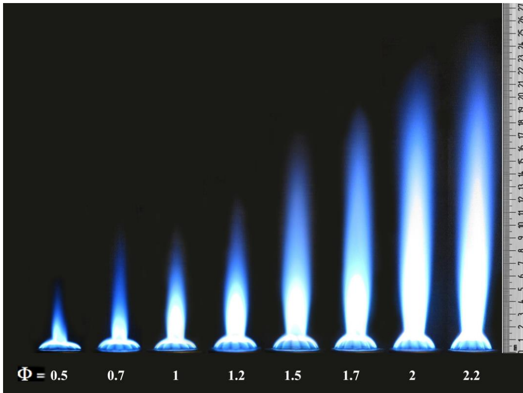
Figure 4.6 LPG with 50% Hydrogen IDF Re=3000
